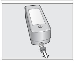
Remove the stoppers from the detergent cartridges.
