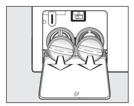
■ Remove the filters completely.
